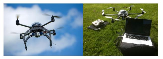
Figure 1 Left: The QuadKopter carrying a video camera. Right: The HexaKopter on the ground with the remote controller and a laptop to set up the system for a GPS waypoint flight.
