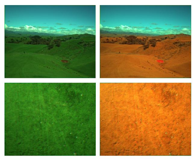
Figure 2 Top left: An RGB image acquired with the Tetracam MCA over a Sheep and Beef farm near Taihape. Top right: Identical image visualised with a near infrared band. Bottom left: A downward looking image from the Tetracam MCA of a pasture paddock. Bottom right: Identical image with a near infrared band.
