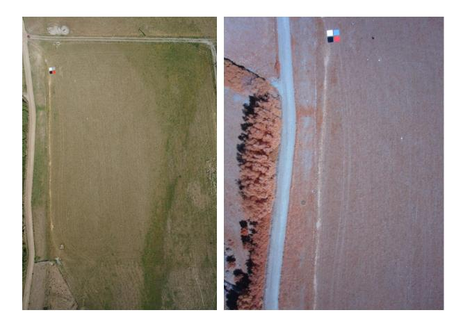
Figure 3 Tarpaulins are used as homogeneous calibration targets for the Empirical Line Method. Left: RGB image of the tarpaulins. Right: Near infrared image of the same area at a lower flight altitude.
