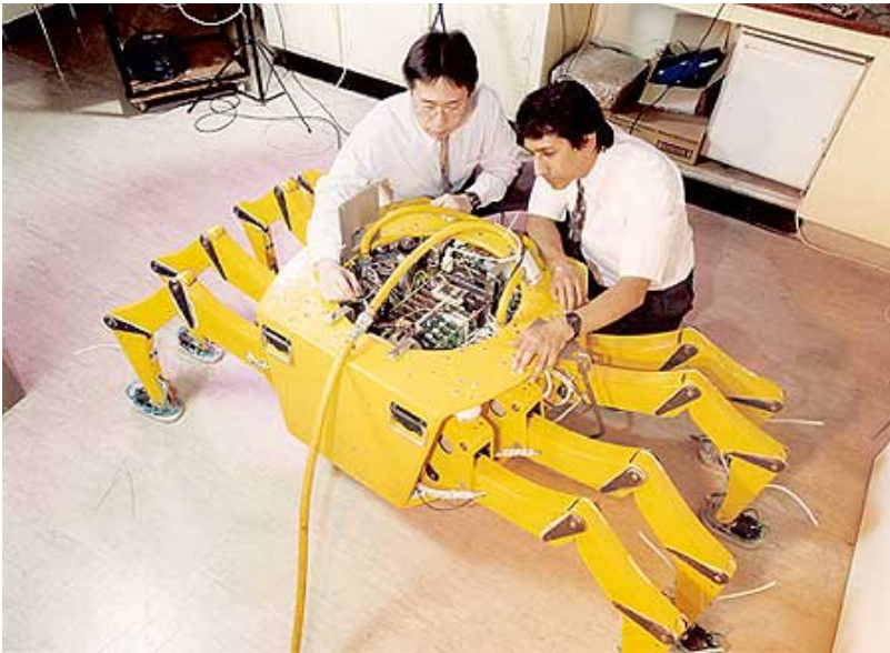
Professor Virk (right) and a colleague with the Robug 3, a robotic climbing spider he helped design and build when he worked in England more than a decade ago.
