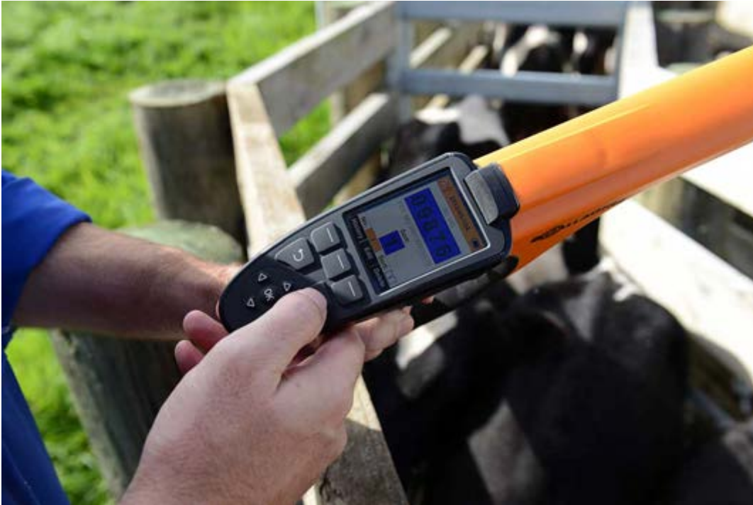
The hand-held reader (HR4), which allows farmers to scan individual livestock identification details from an ear tag
