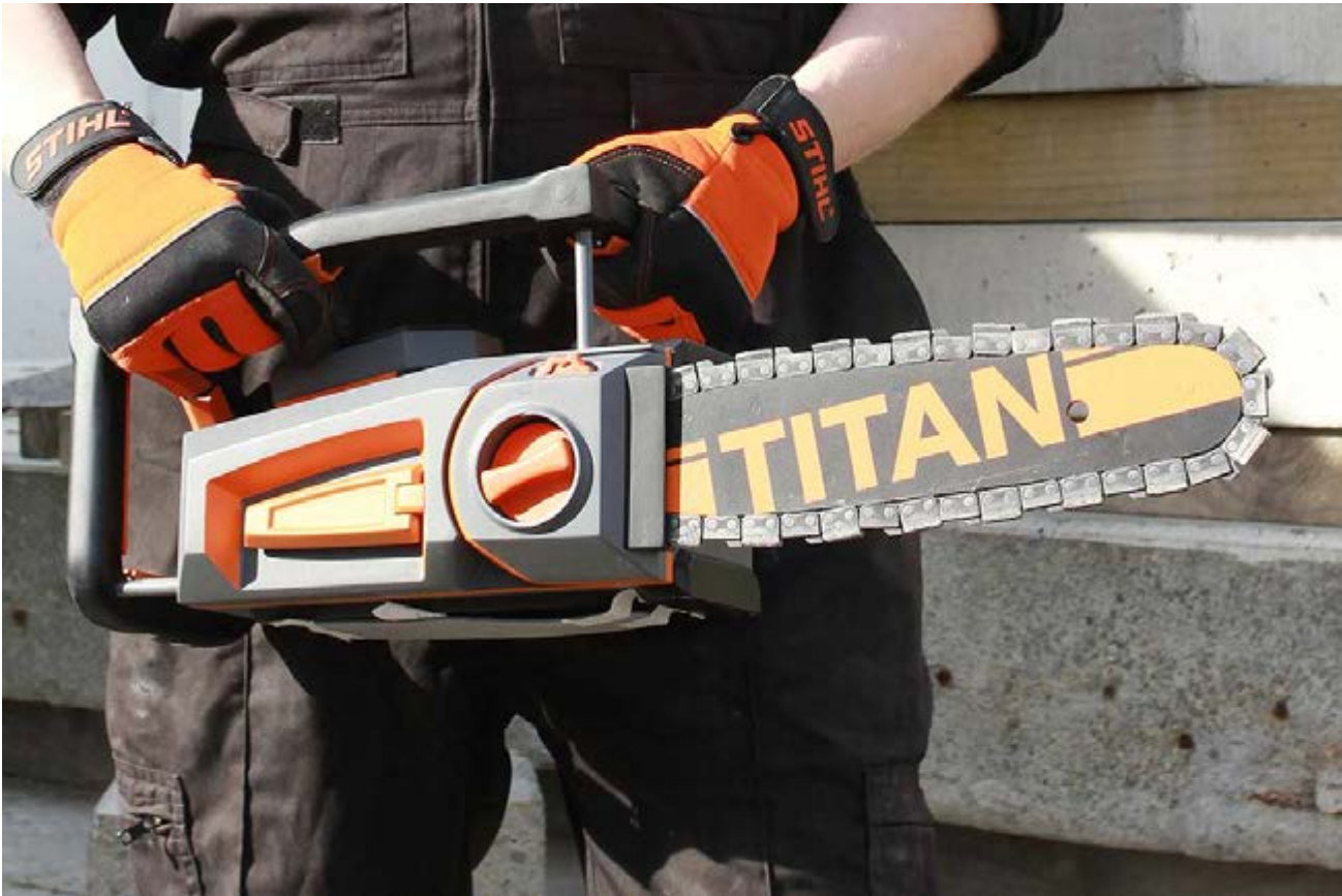
A new purpose-built concrete cutting chainsaw.
