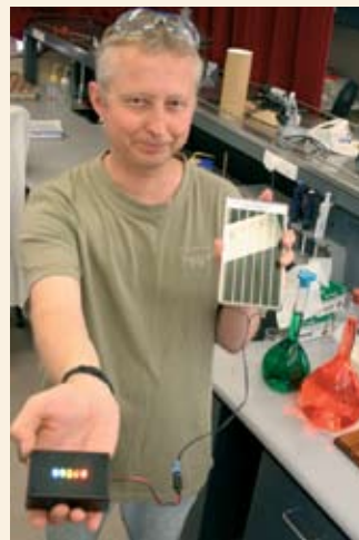
Dr Wayne Campbell holds up a working example of a photovoltaic cell powered by a Massey-developed dye. The cell itself has been engineered by Dyesol, an Australian firm with a licence to manufacture Grätzel cells.
