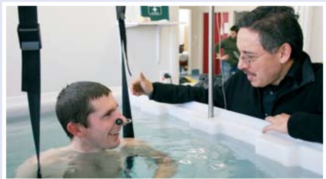
Professor Cunningham, at right, using an underwater weighing tank to determine lean and fat body mass.
