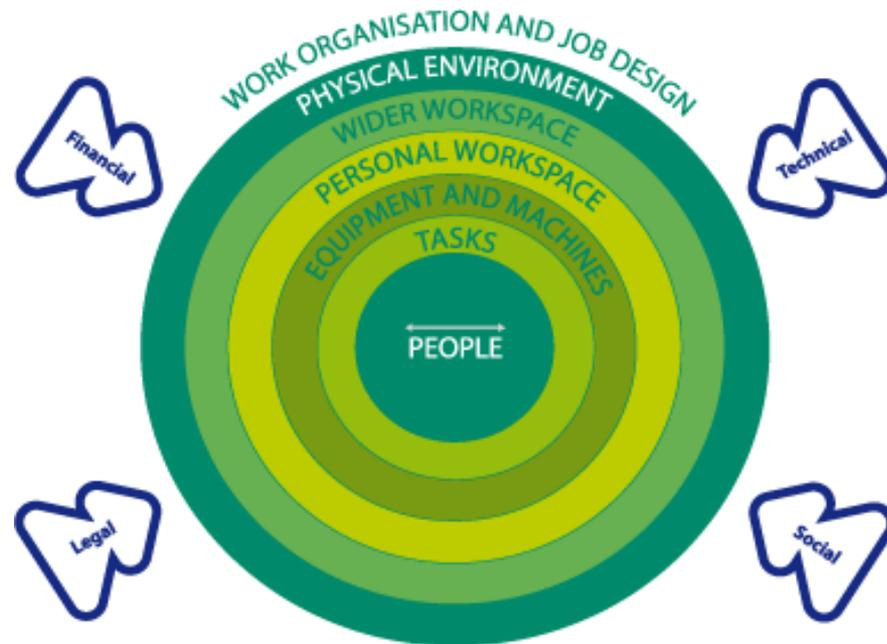
'Concentric Rings' - Model of ergonomics factors relevant to work design.
