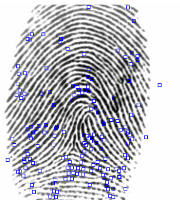
Figure 9: 163 remaining keypoints after the removal of the candidate keypoints with low contrast.
