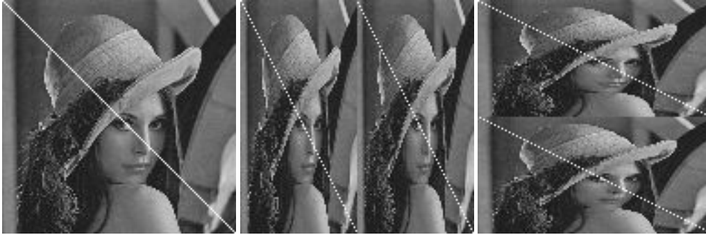
Figure 8. Our initial image of Lena (left) and the image crinkled with a step size of n = 2 in dimension i = 0 (middle) and i = 1 (right). Note the one-pixel width line superimposed over the image, this shows how some pixels are split by the crinkling. This image is arranged as a simple [128][128] image, this resolution was purposely chosen so that the individual pixel data can be clearly seen.
