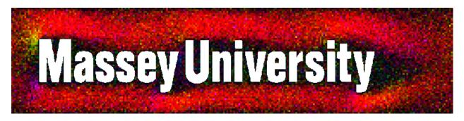
Figure 4: The Lattice Gas Cellular Automata simulating fluid flow past the "Massey University barrier". The cells are coloured using the HSV colour model with hue defined by the direction of the flow and the brightness determined by the velocity.
