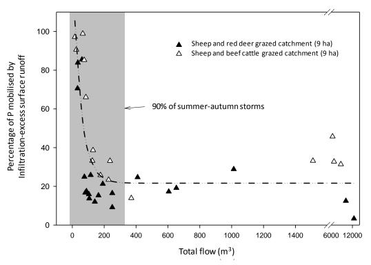
**Fig 3**. Graph showing the proportion of P contributed by infiltration-excess surface runoff decreases with increasing streamflow as saturation-excess and storm sizes increase. The grey box represents the area where 90% of the summer and fall storms occurred.
