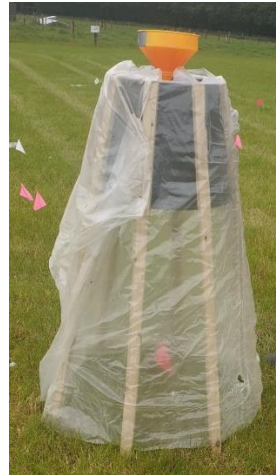
Fig. 1 - Modified frame with funnel designed to mimic a natural urination event
