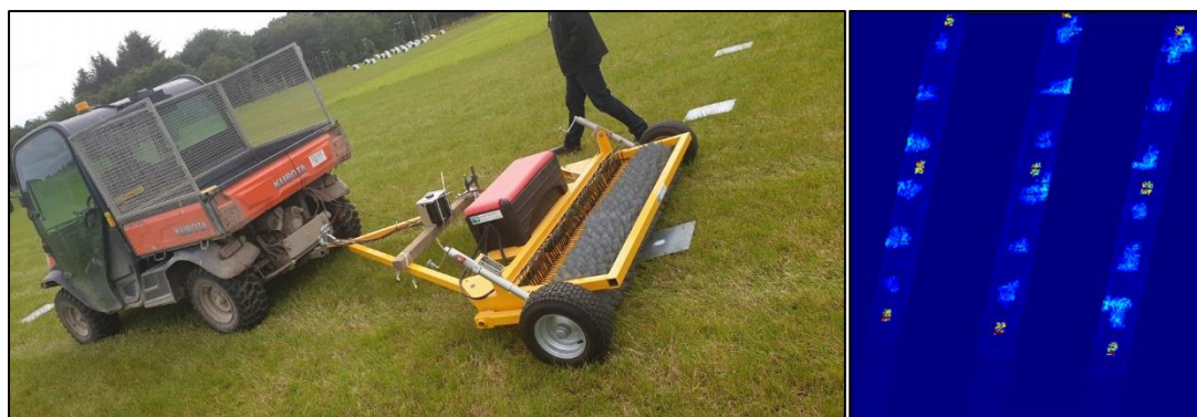
Fig. 4 - Spikey-R instrument towed behind the Kubota vehicle over each metal GCP (left) and (right) the processed PNG files of three side-by-side Spikey-R runs on the wet soil 2 hour simulated urine deposition, illustrating each urine patch (light blue) and GCP (red/yellow/green) against the background pasture.
