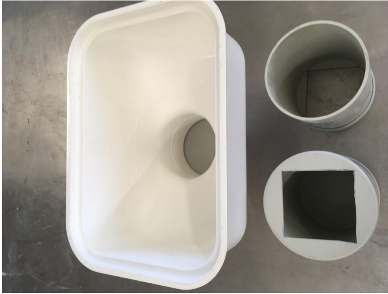
Figure 1: Three different devices for testing lime samples: scale model hopper made from PVC downspout (left) and two cylinders for testing flow from top and bottom.
