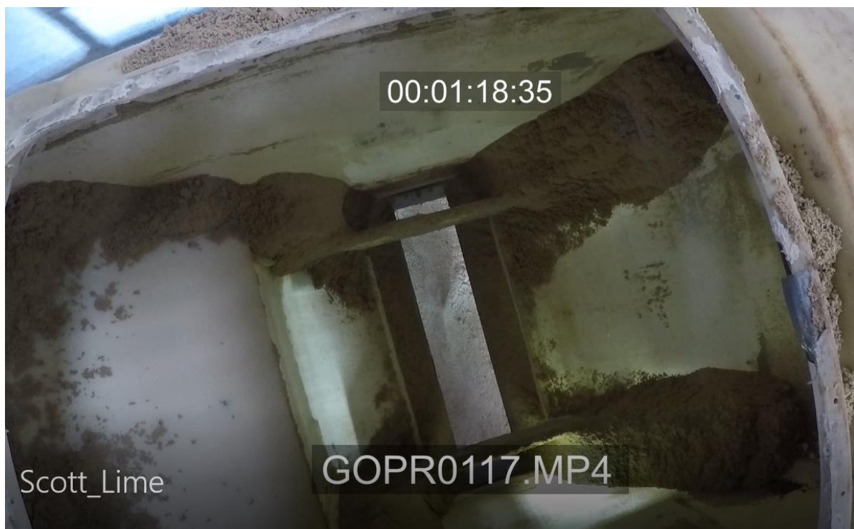
Figure 4: Screen shot of residual lime in hopper for highest moisture level tested (10%) with Webster's lime.
