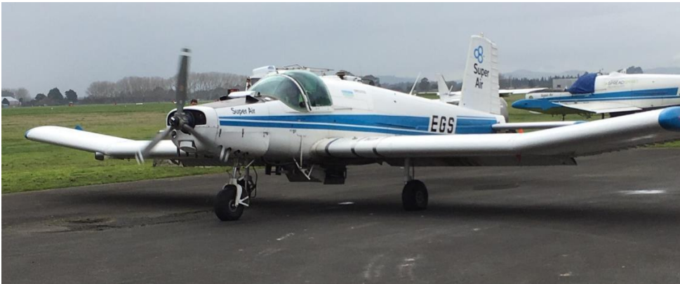
Figure 3: SuperAir plane in Hamilton with 1.2 tonne hopper used for testing.
