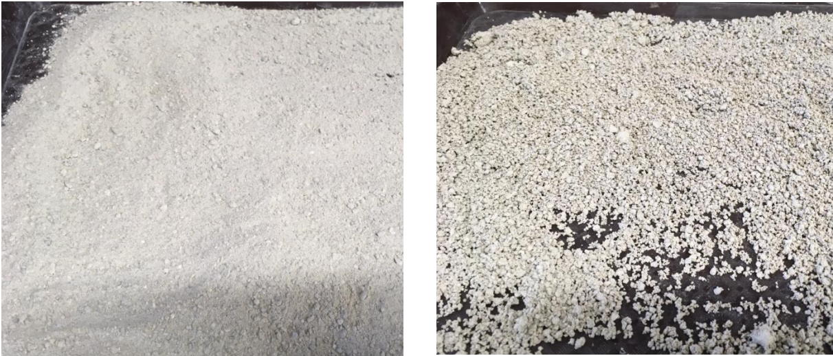
Figure 73: Samples of Supreme lime (left) from before start of testing, and (right) after testing.
