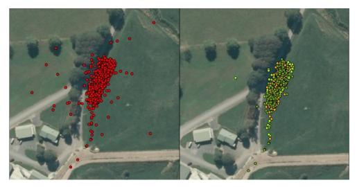
Figure 4: Comparison of noisy (left) and filtered (right) animal location data (Pletnyakov et al., 2019).
