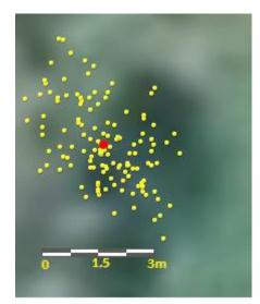
Figure 5. GPS noise while lying down while ruminating (yellow) at a fixed location. The mean estimated position is shown in red (Pletnyakov, et al., 2019).
