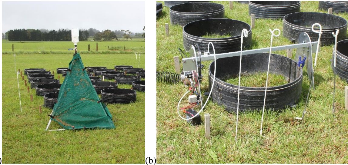
Figure 1. Apparatus used to (a) apply urine patches; (b) apply inhibitor solutions.
