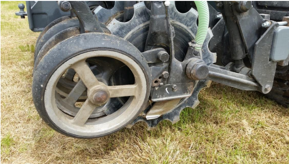
Figure 3. Close-up showing one half of the upside down cross-slot T. The green tube delivers seed and black tube Respond ® to the cross-slot.
