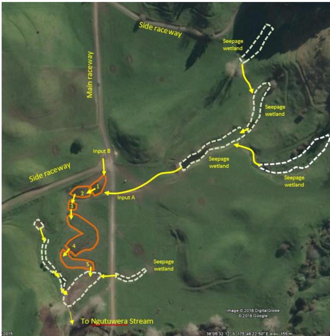
Figure 1. Layout of constructed wetland along with major inlets and outlets. The five monitored constructed wetland cells are defined with orange unbroken lines. Unmonitored wetland cells (constructed and natural seepage) are outlined in broken white lines. Laneways that contribute to the laneway input are identified. W1-W4 are the groundwater sampling wells.
