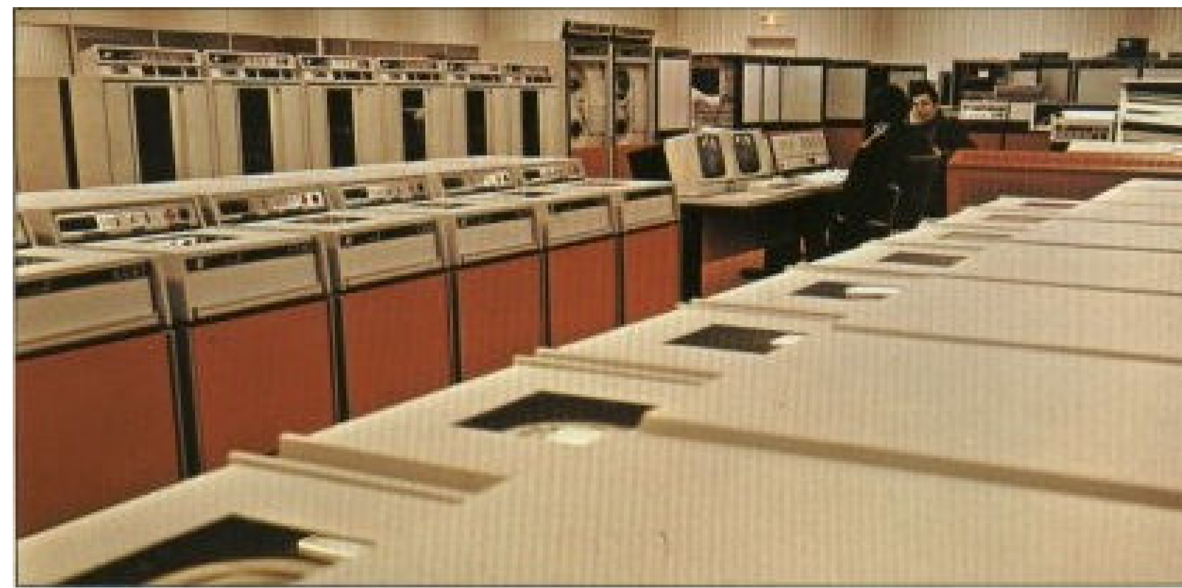
Figure 4: ICL's Distributed Array Processor (DAP) occupying a whole machine room.
