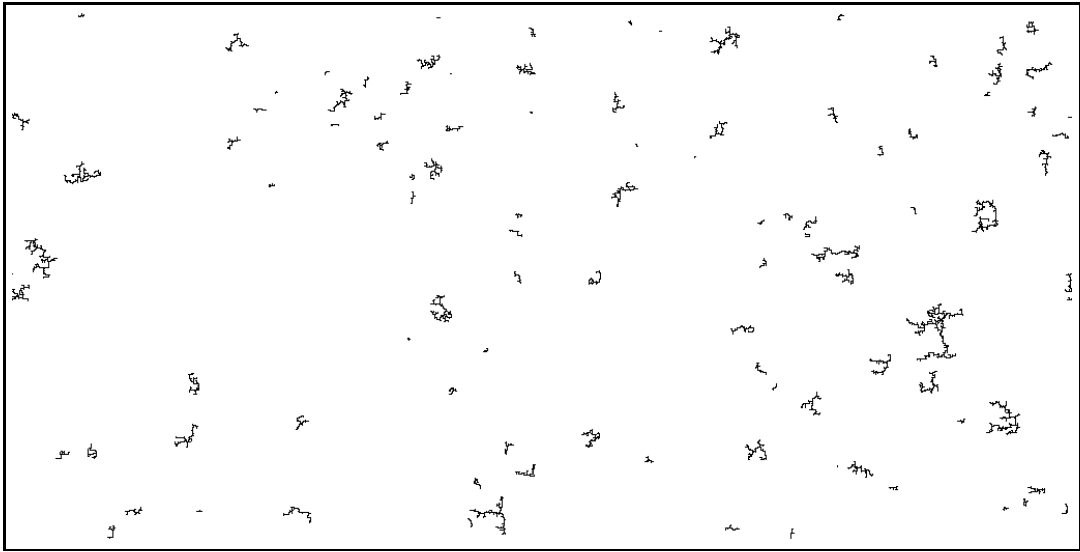
Figure 9: Snapshot of our system at simulation time 508 when run with Peclet number of 1.0. A right to left drift force is applied, which biases the random choice of particle movement.
