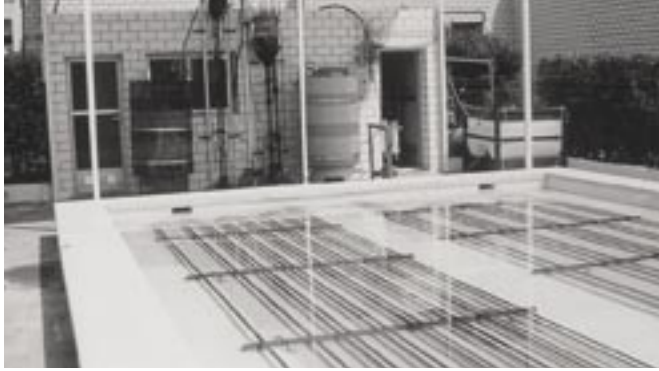
At Almería in Spain a pilot photobioreactor cultures a microalga which will be harvested and processed to produce EPA, a valuable omega-3 oil. Although the extraction process – shown below – is sophisticated and costly, for high-value products the use of photobioreactors is approaching commercial viability.
