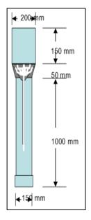
After installation, the top of the fluxmeter sits at a depth of 1 metre below the soil surface, well below the cultivation management zone. Once the soil has re-settled, it will have no influence on the soil management for the crop above.
