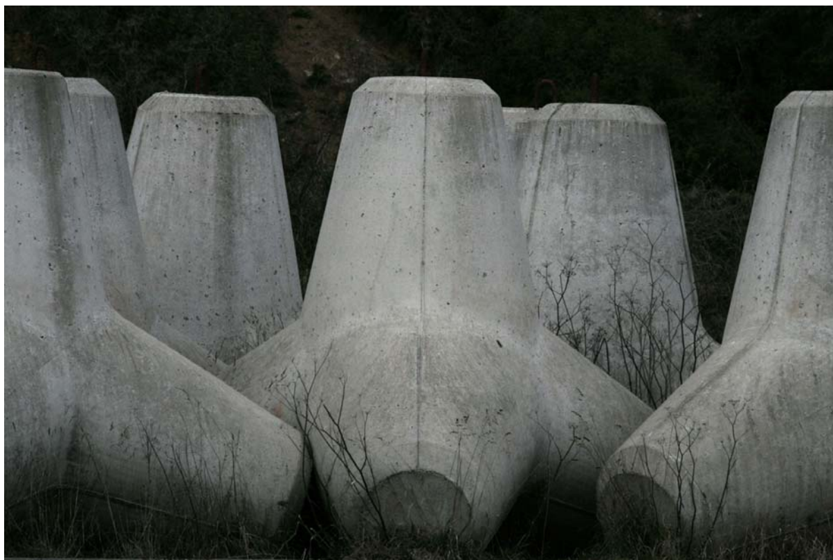
Figure 13: Concrete tetrapods are manufactured in bulk in the old Harbour Board quarry, near the penguin viewing area at the end of Waterfront Road, Oamaru. Photo: I.M Turnbull, 26 July 2007.
