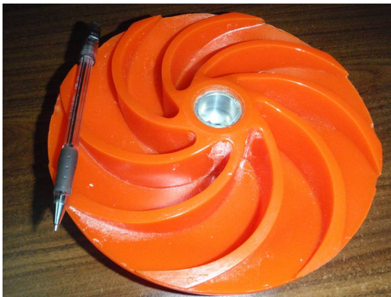
Figure 3.7 Sludge pump propeller of the same type that suffered severe abrasional damage from volcanic tephra.
