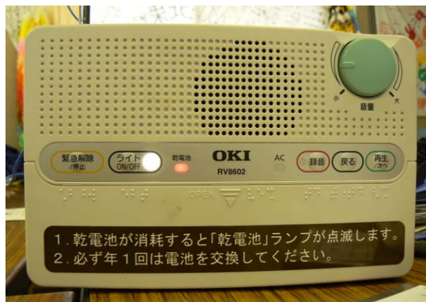
Figure 32 A wireless receiver shown by civil protection officials in Minami-Sanriku. These units are rented by the local government to every household in the town, and resulted in effective warning dissemination on March 11 th 2011.
