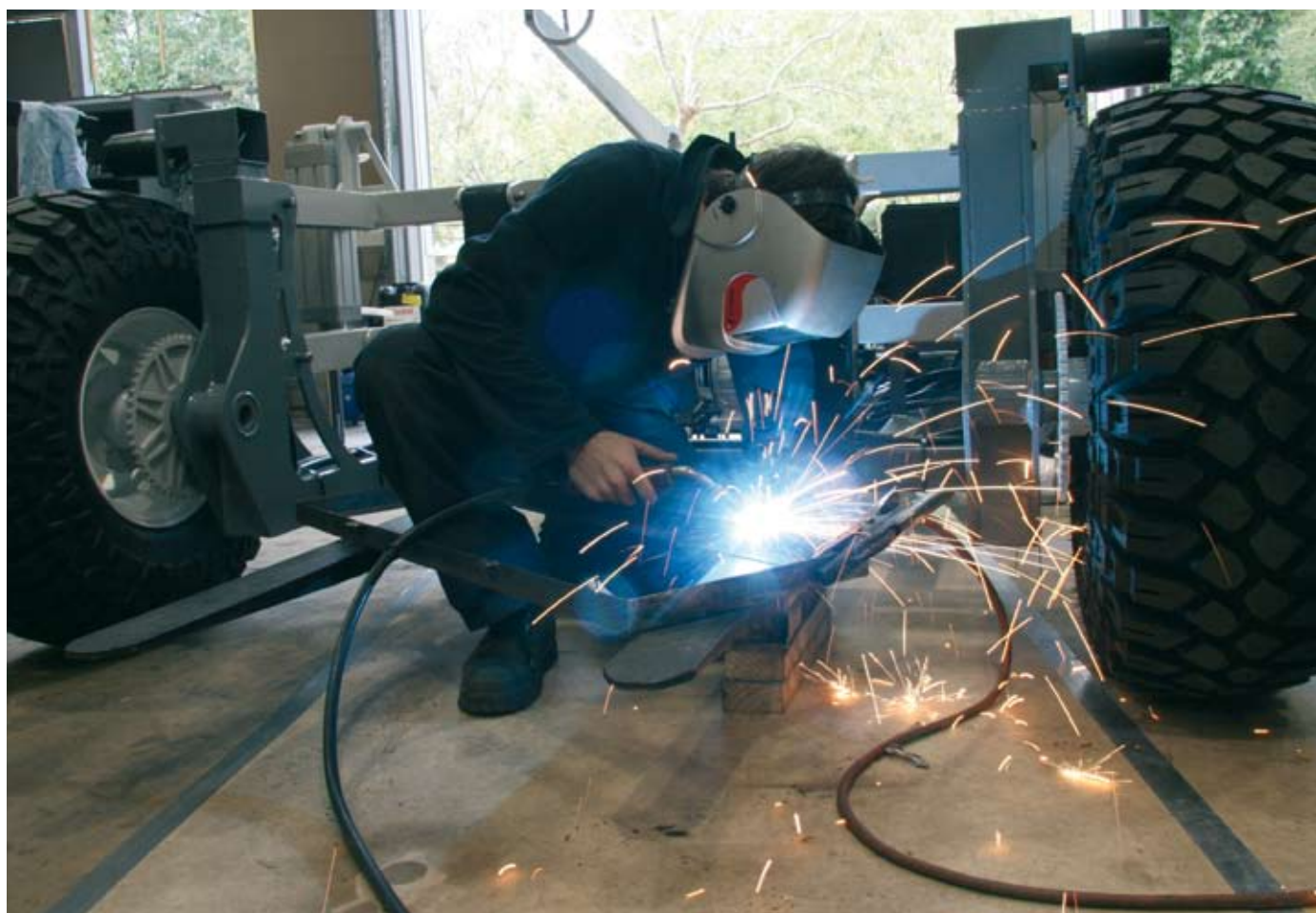
Alistair Scarfe uses an arc welder on the forks that carry the picker's bin. The picker will be powered by either a generator or the low-carbon-footprint option of a rechargeable battery. The controller is quad-core-chipped computer – a high-end PC – running the open source operating system Linux. Like the computer and generator, the cameras and electric motors are also off-the-shelf. What won't be off-the-shelf are the picking arms, each of which will work in three axes. Arms like these are commercially available, but the team will fabricate these themselves at a fraction of the cost. Also being assembled is the base station that the pickers will interrogate remotely whenever instructions are needed. It is the base station that will coordinate the picking paths when two or more pickers are in action. Once the prototype is perfected, the fabrication of the more specialised parts (but not of the final assembly) is likely to be outsourced to local manufacturers. The Massey-designed pickers and packers (see page 24) will be owned by an independent commercial enterprise, which will lease them to industry.
