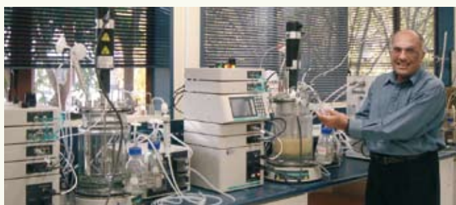
Professor Yusuf Chisti stands alongside two newly commissioned bioreactors. The bioreactors and their PC2-level containment facility complement recently-acquired equipment for recovering biological products. Professor Chisti is researching the use of biocatalysts – biotech microorganisms, animal and plant cells, enzymes, and subcellular components – to produce novel bioactive substances, vaccines, potential therapeutics, diagnostic antibodies and other high-value products.
