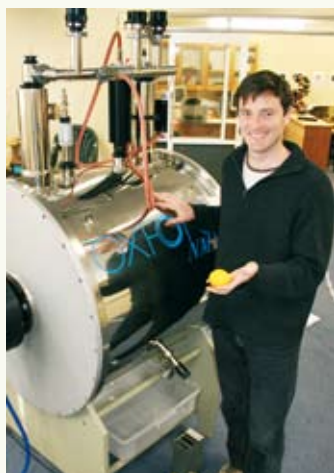
Riddet Centre researcher Dr Jason Hindmarsh stands alongside an MRI machine which he and Institute of Fundamental Sciences researcher Robin Dykstra have re-commissioned. The machine will be used to track how the composition of a mix of milk and probiotic bacteria changes as it is dried and rehydrated.
