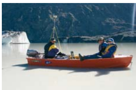
Two boats were used in the survey of the Tasman's lake, one (upper photo) carrying an echo-sounder to measure lake depth, the other (lower photo) pulling a towfish sonar, imaging the sub-bottom materials beneath the lake floor. The towfish sonar, a shallow seismic technique, is used to identify subsurface ice and the sub-bottom sedimentary stratigraphy.
