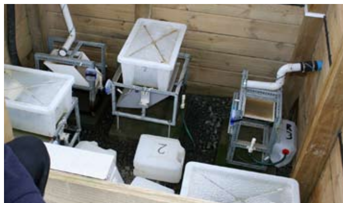
An effluent drainage monitoring station used on Massey's No 4 Dairy Farm near Palmerston North
