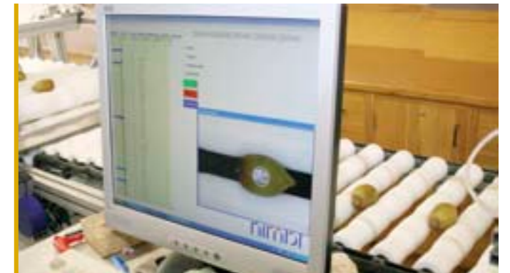
A packing robot developed using artificial vision was designed to sort and pack up to 400 trays of kiwifruit per hour, but the machine will first become operation in the apple industry this harvest.
