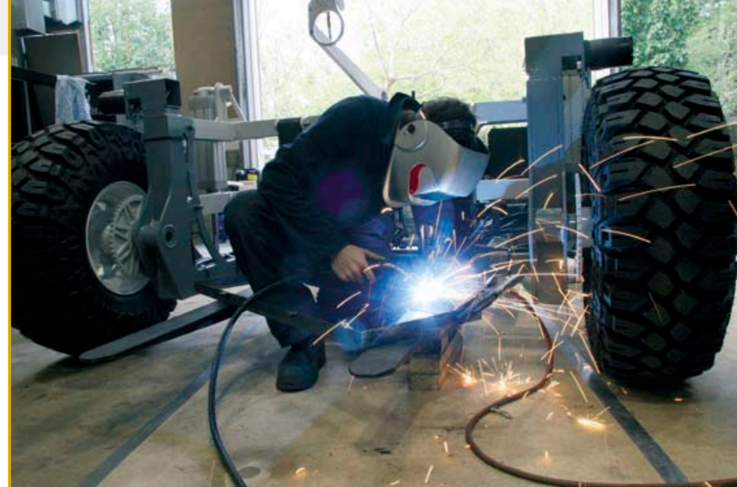
Alistair Scarfe uses an arc welder on the forks that carry the picker's bin.
