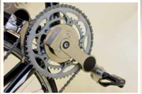
The state-of-the-art cranks used to gather force data
