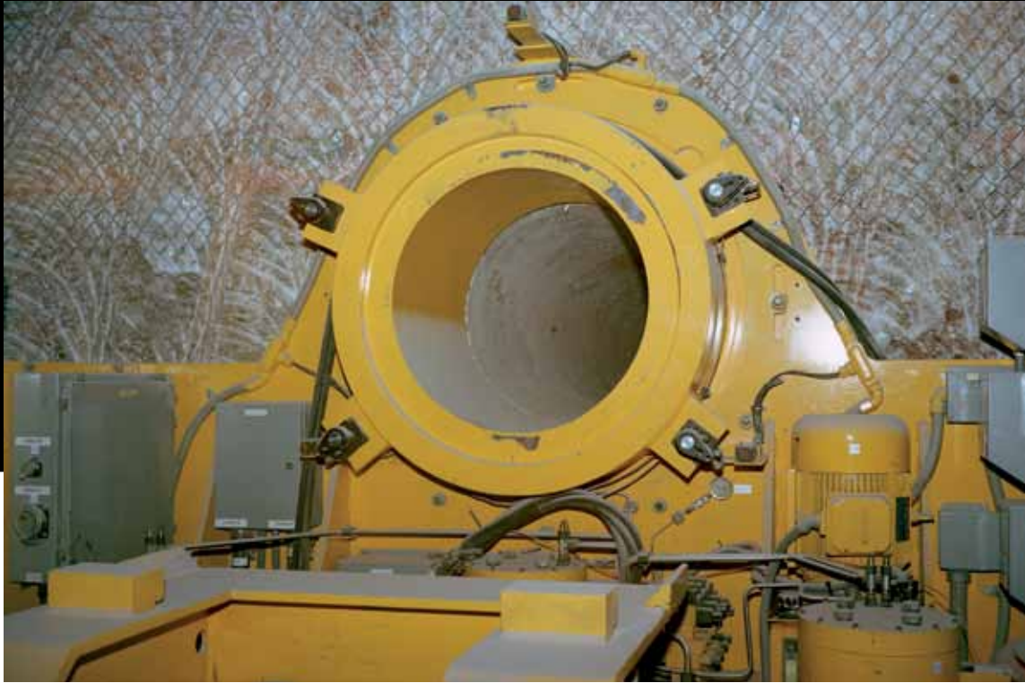
Transuranic waste remote handling insertion machine (underground salt walls), Waste Isolation Pilot Project, New Mexico, USA 2006
