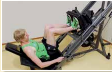
A modified leg press allows for precise control of the load and type of contraction used during exercise by way of an automated hydraulic system.
