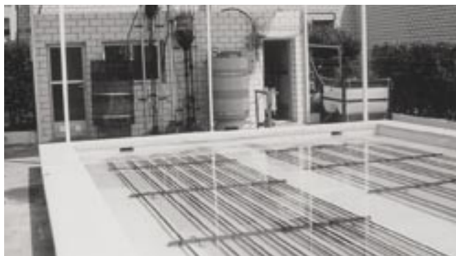
At Almería in Spain a pilot photobioreactor cultures a microalga which will be harvested and processed to produce EPA, a valuable omega-3 oil. Although the extraction process – shown below – is sophisticated and costly, for high-value products the use of photobioreactors is approaching commercial viability.
