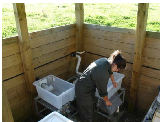
Figure 5.2.6 Drainage water being collected from artificial tile drains installed in a pasture paddock at No. 4 dairy, Massey University, using a tipping bucket method. (Photo: C Christensen).
