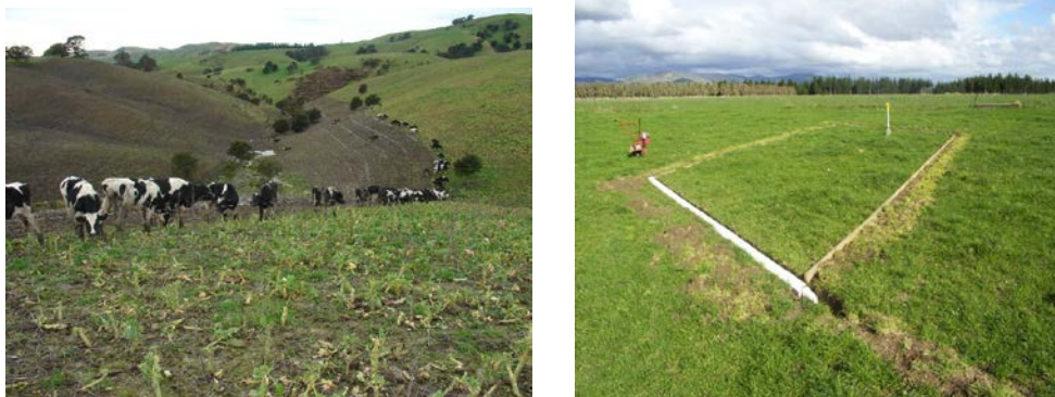
Figure 5.2.7 Examples of sub-catchments (left) and artificial sub-catchment (right) used to measure nutrient loss in surface runoff.
