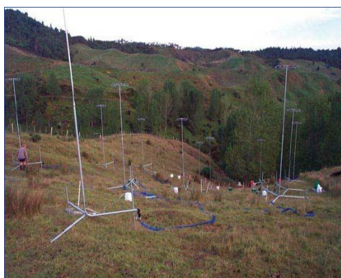
Figure 5.2.8 Large scale rainfall simulation experiment established in the Waikato hill country to measure bacteria loss in surface water runoff (Photo: R Collins).
