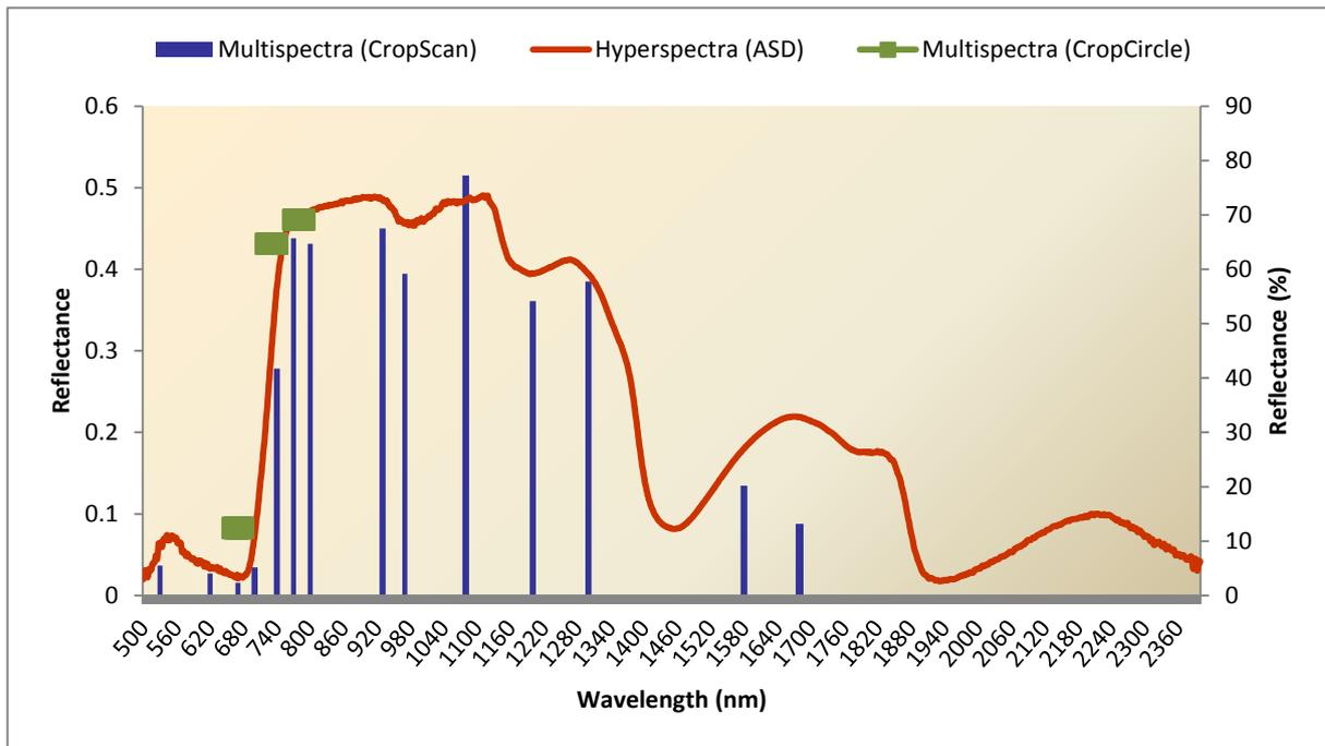
**Figure 1 Pasture reflectance of multispectral (CROPSCAN and Crop Circle) and ASD Field Spec<sup>®</sup> Pro hyperspectral devices.**
