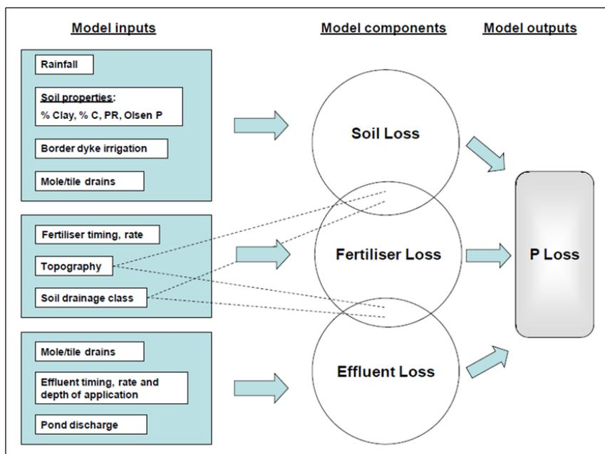
**Figure 1.** Conceptual diagram of model structure.
