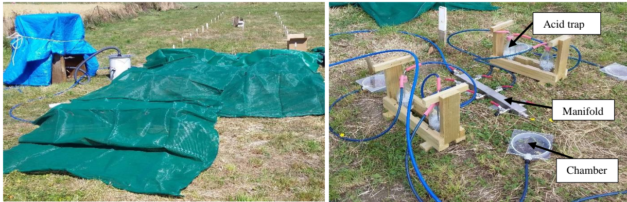
Figure 1: Ammonia sampling site and set up of the Dynamic Chamber method
