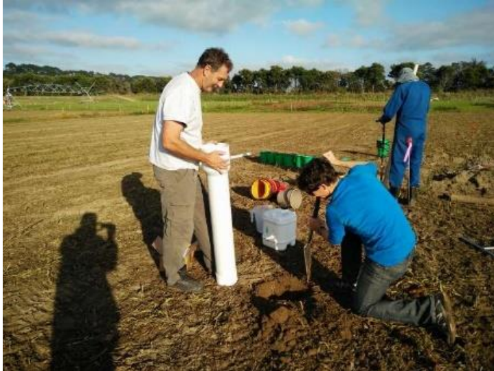
Fig. 2 Installing the flux meters. Once the DFM was inserted into the hole, the soil was repacked layer by layer.
