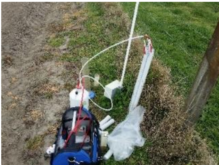
Fig. 3 Pump designed to collect drainage from DFMs
