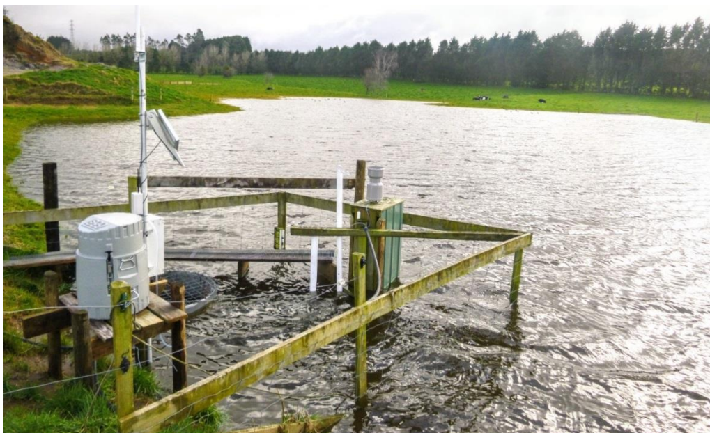
Figure 1: Photo of a pond formed on pasture by a detention bund impeding the flow of surface runoff generated during a storm event. The fencing protects sampling equipment from livestock.
