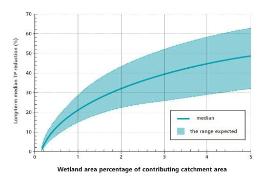
**Figure 2:** Performance estimates for reduction in total phosphorus (TP) based on wetland size. Note that the phosphorus performance estimates do not apply to tile drainage flows or areas with high (more than 35%) clay content in soils.
