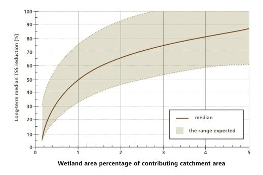
**Figure 1:** Performance estimates for reduction in total suspended solids (TSS) based on wetland size. Note that the sediment performance estimates do not apply to tile drainage flows or areas with high (more than 35%) clay content in soils.
