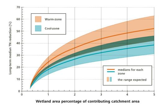
**Figure 3:** Performance estimates for reduction in total nitrogen (TN) based on wetland size and whether situated in a warm or cool zone in New Zealand. Note that nitrogen removal generally decreases as temperature decreases. Different performance estimates are therefore provided for warmer (median annual air temperatures ≥12°C) and cooler (median annual air temperature 8 - 12°C) regions of New Zealand (see Figure 4 in the guidance document).
