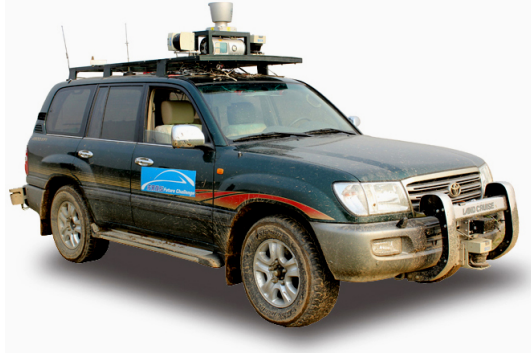
Fig. 6 Our ALV used for the experiments in various environments. It is equipped with some cameras, lasers, and positioning sensor for perception
