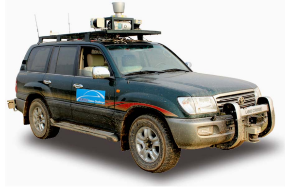
Fig. 8. Our ALV used for the experiments in various environments. It is equipped with a Velodyne HDL-64E S2 LIDAR, a NovAtel SPAN_CPT GPS-aid INS, and some cameras for perception.
