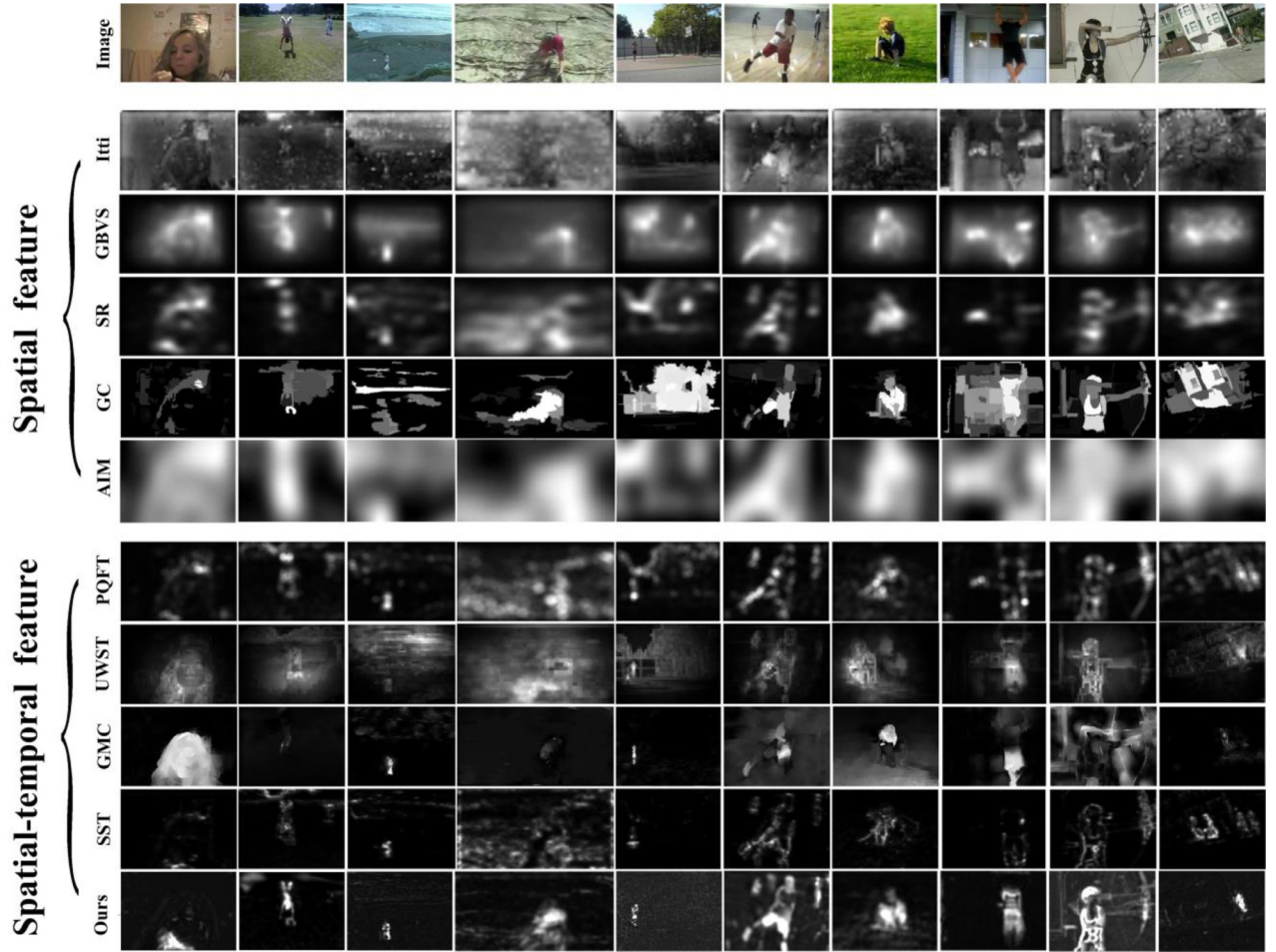
Fig. 2. Qualitative comparison of saliency maps. First row: original images; Second–sixth rows: five typical methods using spatial features; Seventh–last rows: four typical methods jointly using spatial–temporal features and our proposed method.
