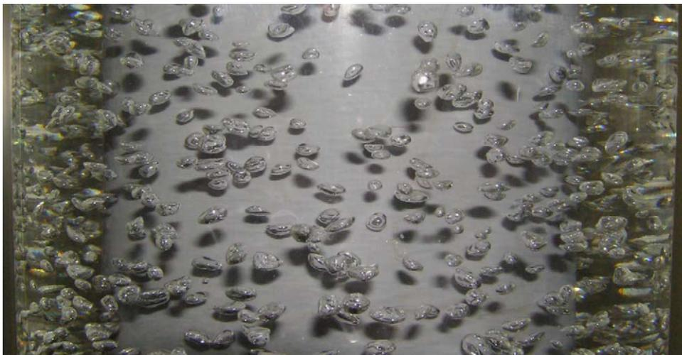
Fig. 2. A typical distribution of bubbles at  $Q_L = 2 \text{ m}^3/\text{h}$  and  $Q_g = 1.29 \times 10^{-4} \text{ m}^3/\text{s}$ .
